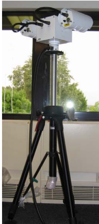
Figure 5.2-1: PTZ controlled platform with visible and IR cameras
