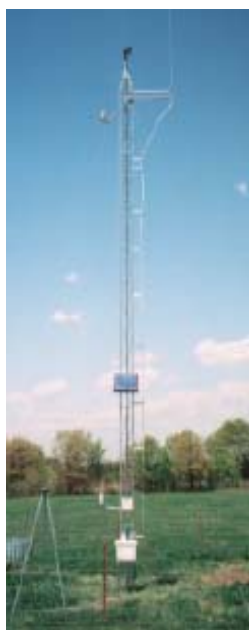
Figure 2.2-2: Installation: Heavy Duty Aluminum tower - Option A
