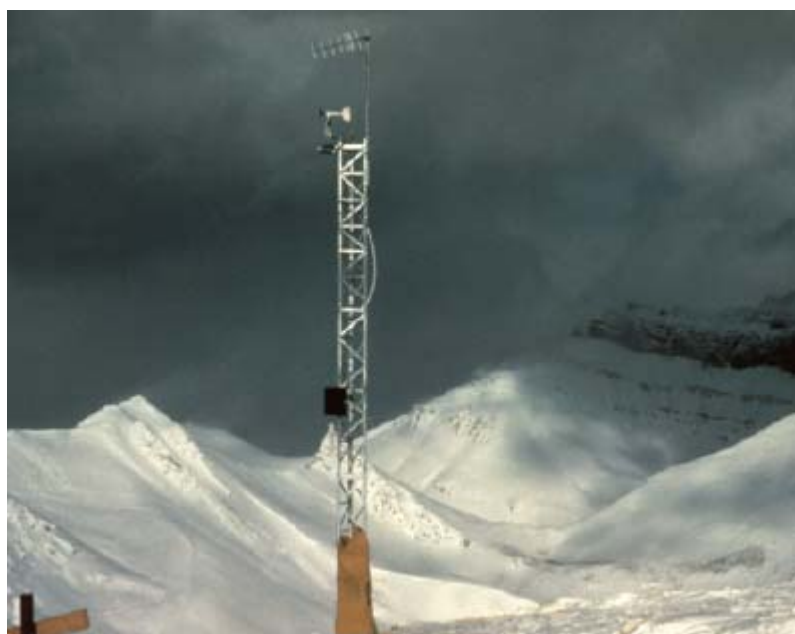
Figure 2.2-2: Installation: Heavy Duty Aluminum tower - Option A
