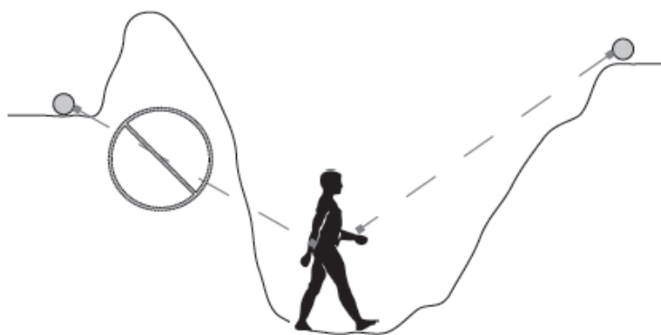
Figure 2.6-19: Surveillance line of sight blockage due to terrain obstructions
