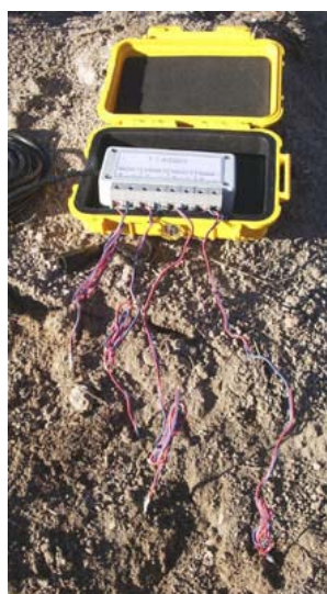
Figure 2.1-15: TTT4 Multi-Sensor thermocouple and wires
