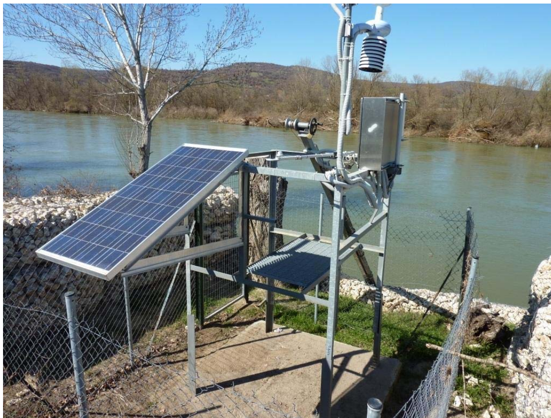
Figure 2.2-3: Installation heavy duty frame – Option B
